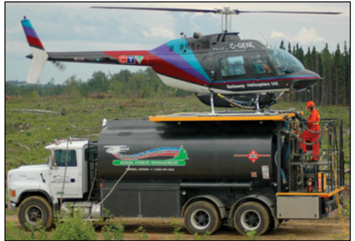
Loading a spray aircraft with modern leak-proof systems and appropriate personal protective equipment.
